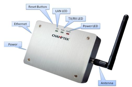
Power LED – On when reader is powered. TX/RX LED – On while reader is transmitting or receiving a packet. LAN LED – Blink when there are network activities. Ethernet – RJ-45 Ethernet jack. Antenna – SMA connector Power – 5Vdc Reset Button – Hardware Reset the Reader
