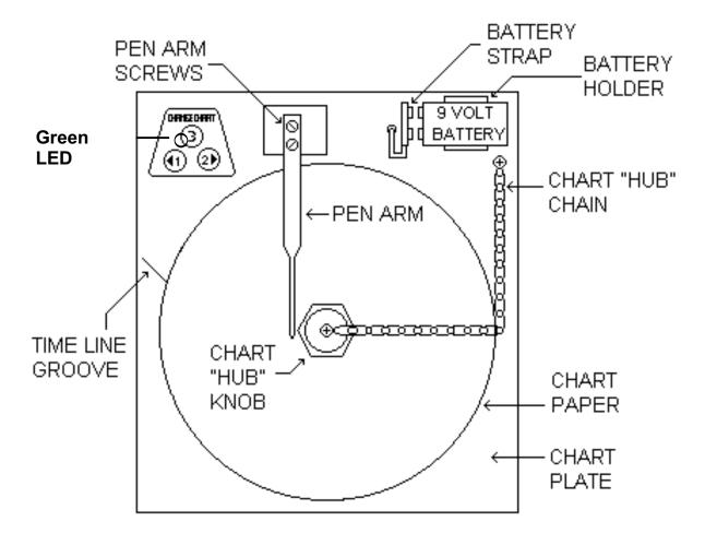
Figure 2.10 Recorder Platen Layout/Battery Installation
