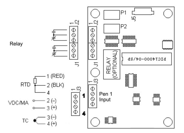
Figure 2.5 Two Pen OEM Ink Style Inputs
