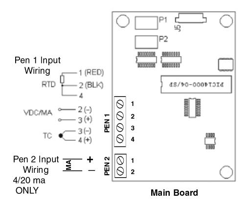
Fig. 2.6 Two Pen Universal and Thermal Inputs
