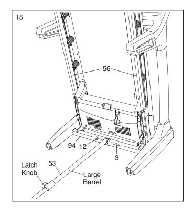
16. Attach the upper end of the Storage Latch (53) to the Frame (56) with a 3/8" x 2" Bolt (3) and a 3/8" Nut (12).
