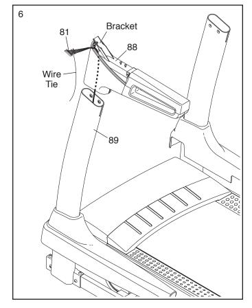
7. Attach the Left Handrail (88) to the Left Upright (89) with two 5/16" x 1" Screws (5), two 5/16" Star Washers (11), and a 5/16" x 1 1/2" Bolt (4). **Do not tighten the Screws and the Bolt yet.**
