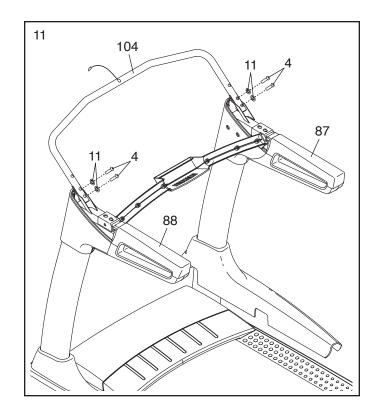
12. With the help of a second person, hold the console assembly near the Left Handrail (88).
