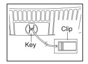
In an emergency, the key can be pulled from the console, causing the walking belt to slow to a stop. Test the clip by carefully taking a few steps backward; if the key is not pulled from the console, adjust the position of the clip.
