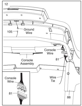
13. Set the console assembly on the Right and Left Handrails (87, 88). **Be careful not to pinch any wires.** Insert the excess Upright Wire (not shown) into the Left Handrail.
