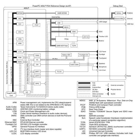
Figure 1: Block diagram of the eLAP
