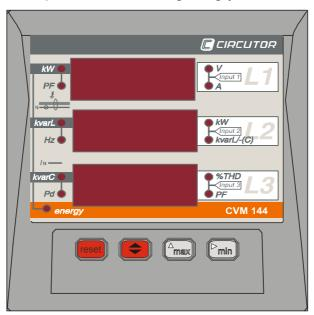
The CVM-144 is an instrument which measures, calculates and displays all the main electrical parameters at any electrical network (balanced or not). The measuring is true RMS value, through three a.c. voltage inputs and three a.c. current inputs (from Current Transformers .../ 5A).
