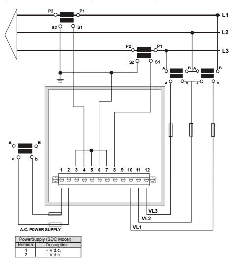
**IMPORTANT REMARK!** If  $\underline{power} = -0.01$  is shown for any of the phases (codes 03, 09 and 15) and voltage and current are not zero for this phase, check out following points:
