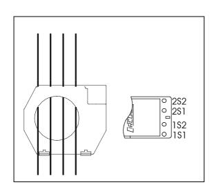
One single WG series transformer can be use for the measurement of residual currents within the range to 3 A or to 30 A, jut depending on the arranged connection diagram.
