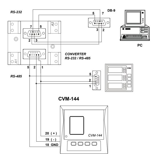
\*If the RS485/232 converter with RTS control ability (code 770208) is used, then the pin 7 connection in the 232 side is not necessary to be done.
