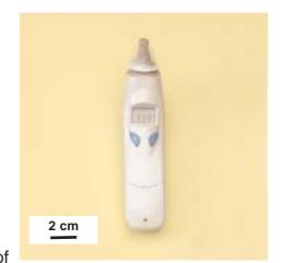
three readings in the same ear for critical situations as variations  $\pm 0.2 \sim 0.3$  °C are to be expected. Beep indicates measurement is complete.
