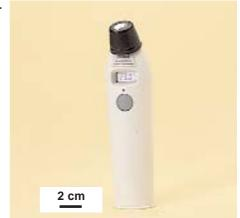
line. Then lift the probe and touch on the neck, moving the probe upwards just behind the ear lobe, and release the button to read the temperature. Core (arterial) body temperature is displayed if the temperature is between 34.5°C to 42°C. Outside this range the skin surface temperature is displayed. Keep the lens clean
