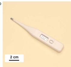
(four beeps). Switch off to conserve battery. Clean before and after each patient measurement. Factory set display units, either °F or °C.
