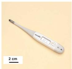
ously and a flashing 'C' is displayed. Audible tone (10 beeps) when temperature rise is > 0.1 °C in 8 seconds. Turn off by pressing the on/off button again. Replace thermometer when 'ERR' is displayed.
