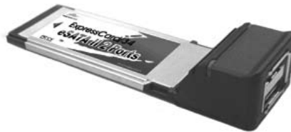
Figure 2-6, PCIe adapter card that supports an external SATA interface in a notebook.
