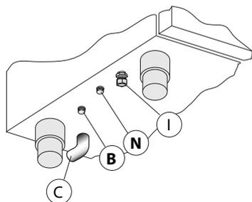
C - Water drain manifold
