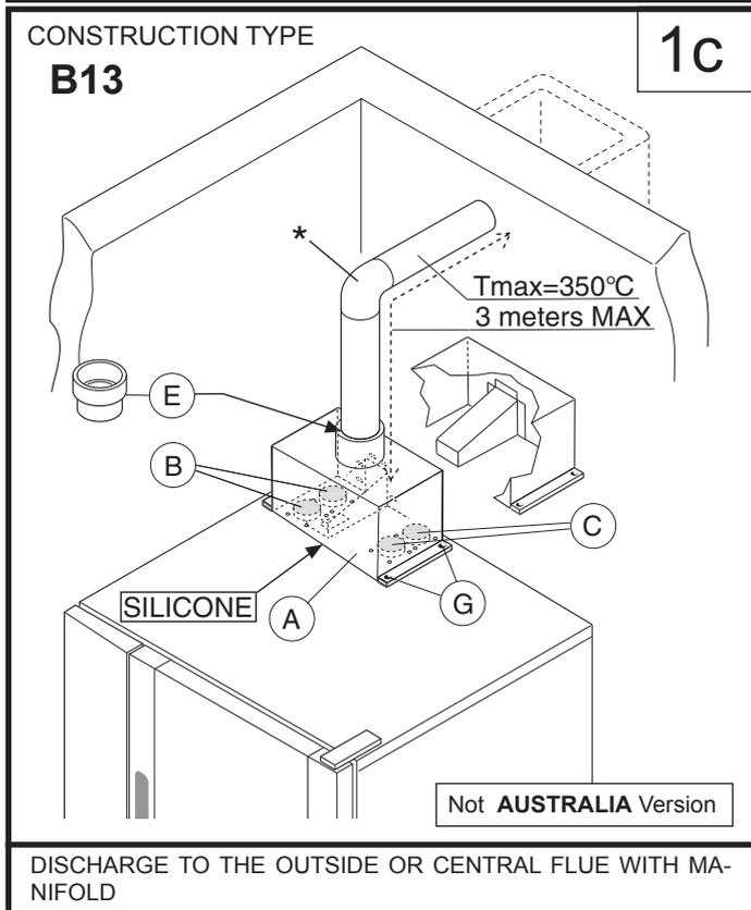
b) choose the diagram with the type of construction from those given below, depending on how the burnt gases are to be exhausted from the place of installation (e.g. discharge under extraction hood, to the outside or to a central flue).
