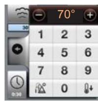
keypad for adjusting the core probe temperature
