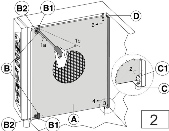
To refit the wall, repeat the steps in reverse order and retighten nut C1.
