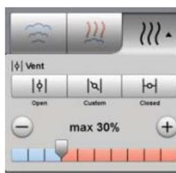
**Humidity setting and adjustment :** for activating or excluding the humidity or adjusting the required level in the **Hot Air Cycle**.
