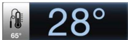
**Digital thermometer/thermostat** for control of product core temperature.
