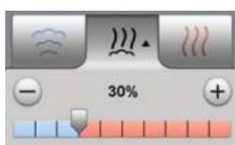
**Electronic humidity adjustment** for adjusting the required humidity level in the **Combi Cycle**.
