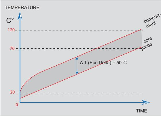
The graph shows an example with a set Delta of 50°C where the compartment temperature increases, keeping this difference of 50°C constant with respect to the core probe. This type of cooking is slower than the conventional cooking method but has the advantage of obtaining better product results and quality. This type of cooking is ideal for large pieces of meat.
