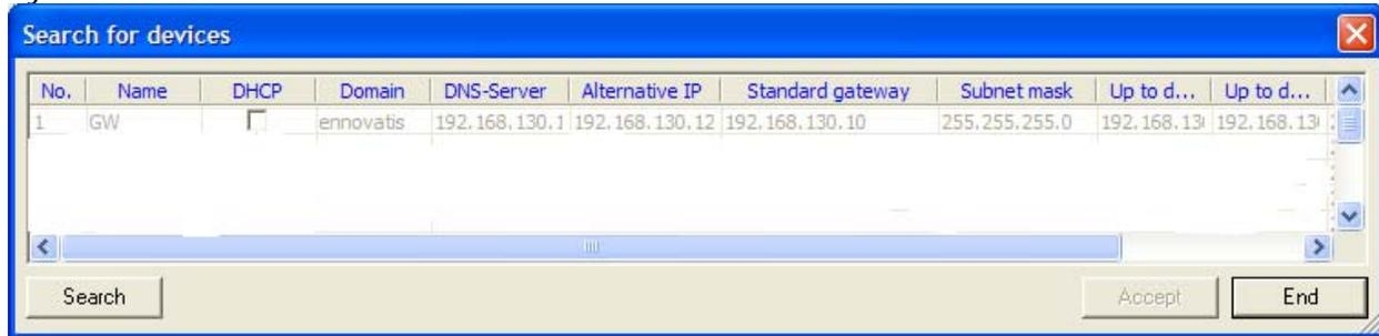
Found devices can be marked and transferred directly to the building. In addition to this, network data such as TCP/IP addresses of devices which have been found are displayed.
