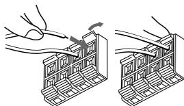
For each speaker (except for subwoofer), connect one end of the speaker signal cable (not supplied) to the speaker terminal on the rear panel and the other end to the speaker. (For connecting a subwoofer, see page 7.)
