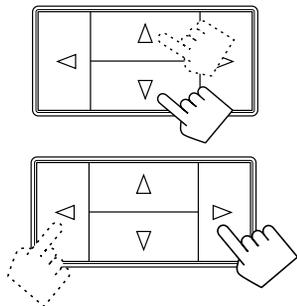
6. Press Control  $\Delta / \nabla$  until “-DELAY +” appears on the display.
