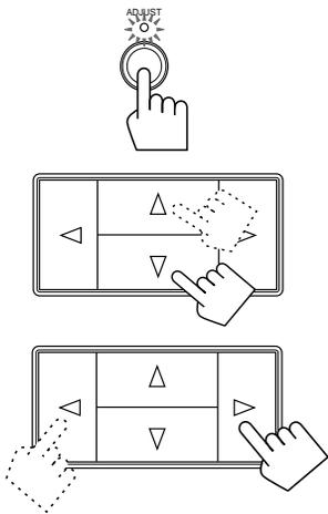
3. Press **ADJUST** so that the Control  $\Delta$  /  $\nabla$  /  $\triangleleft$  /  $\triangleright$  buttons work for surround settings.
