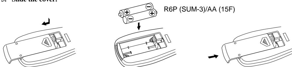
If the range or effectiveness of the remote control decreases, replace the batteries. Use two R6P (SUM-3)/AA (15F) type dry-cell batteries.
