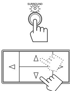
1. Press SURROUND so that the Control  $\Delta$  /  $\nabla$  buttons work for selecting the surround modes. The lamp above the button lights up.
