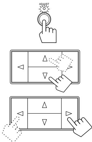
3. Press ADJUST so that the Control Δ / ▽ / ◀ / ▶ buttons work for adjusting the selected surround mode. The lamp above the button lights up.
