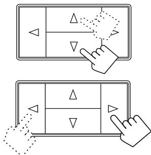
8. Press Control  $\Delta / \nabla$  until “TEST” appears on the display, then press Control  $\triangleleft / \triangleright$  to start checking the speaker output balance.
