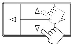
1. Press **PRESET SEA** so that the Control  $\Delta / \nabla / \triangleleft / \triangleright$  buttons work for preset SEA setting. The lamp above the button lights up.
