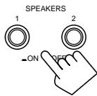
**To use the set of speakers connected to the FRONT SPEAKERS ① terminals**, press SPEAKERS 1 to set it in the **⬇️ON** position, and press SPEAKERS 2 to set it in the **⬆️OFF** position.
