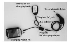
Note: You can charge both PDA and the spare battery at home by plugging the PDA AC charger (comes with your PDA) instead of the car charger into the DC charging adapter.
