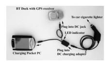
Note: You can charge both PDA and iGPS-BT at home by plugging the PDA AC charger (comes with your PDA) instead of the car charger into the DC charging adapter.
