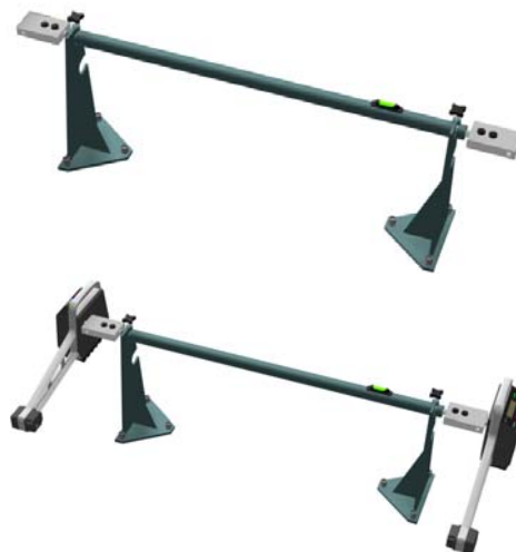
Fig.3.9 Calibrating frame and its converter connector
