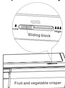
●The humidity control adjusts the airflow in the crisper; higher airflow results in lower humidity. Slide the humidity control to the right in order to increase humidity.
