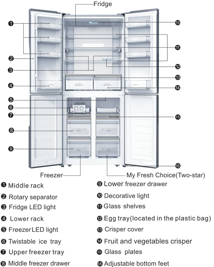
**Note:** Due to unceasing modification of our products, your refrigerator may be slightly different from this instruction manual, but its functions and using methods remain the same. To get more space in the freezer, you can remove drawers (except lower freezer drawer) and twistable ice tray.
