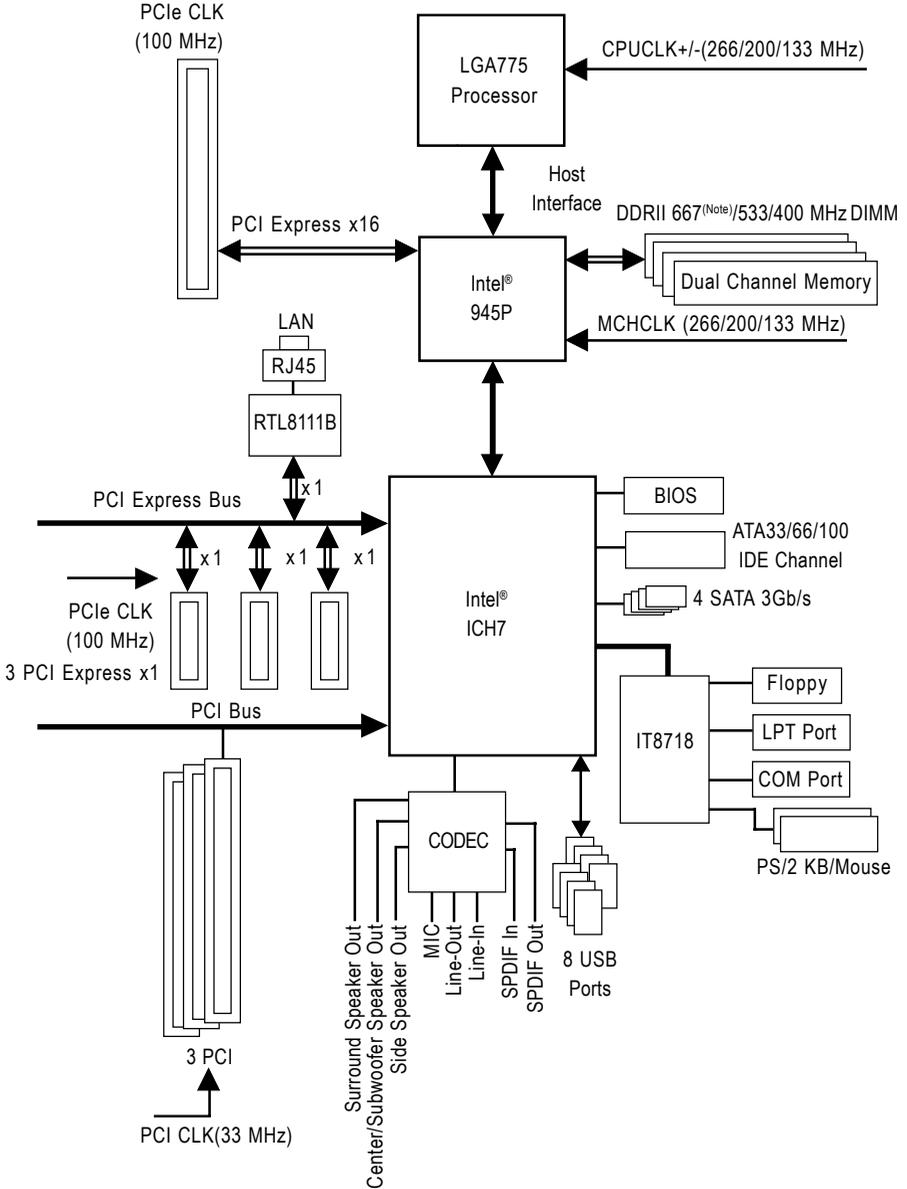
(Note) To use a DDR II 667 memory module on the motherboard, you must install an 800/1066MHz FSB processor.
