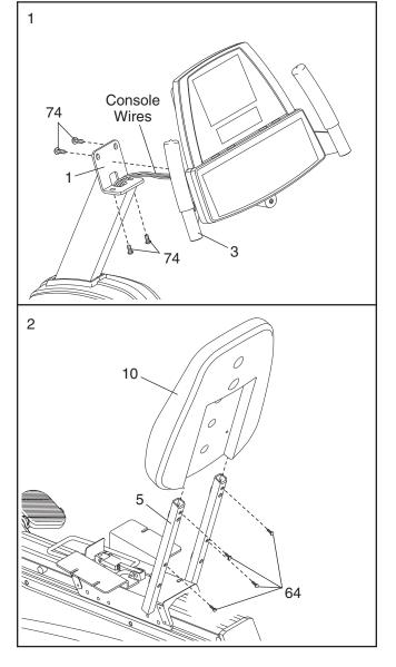
2. Attach the Seat Back (10) to the Seat Carriage (5) with four 1/4" x 3/4" Socket Screws (64).
