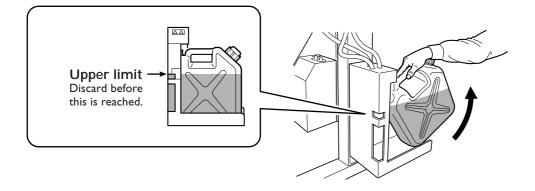
$\boldsymbol{3}$ . Attach the emptied bottle and reset the discharged-fluid count.
