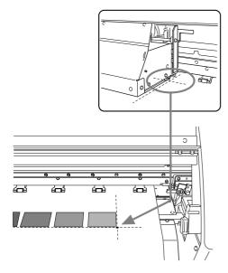
Holding down **(EST PRINT)** for one second or longer prints a test pattern. You can print the test pattern where you want by using **(V)** to move the print heads, then pressing . The front cover may be open during movement, but be sure to close it before you press **(EASE FONT)**.
