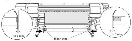
**2** Adjust the positioning of the slider unit to match the width of the media.
