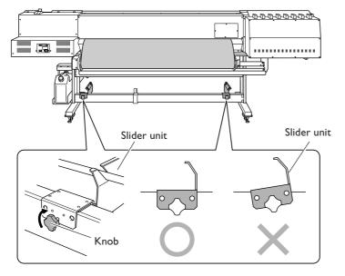
4 Pass the tracking shafts through the looped media and fit then into the grooves of slider unit (right and left).
