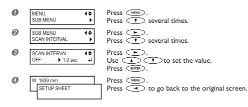
You use this when ink dries poorly. Larger values produce progressively slower movement of the media, enabling you to extend the drying time accordingly. Printing time takes correspondingly longer.
