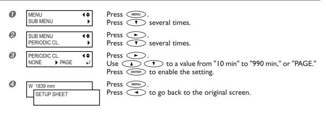
Ink tends to collect on the surface of the heads when you use media prone to build up a static charge, when the ambient temperature is low, and at other such times. Under some conditions, this ink may be transferred to the media. Use this feature at such times. The ink buildup is removed as printing is performed.
