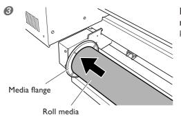
Fit the hole of the roll media all the way onto the left-hand media flange. Press in all the way.
