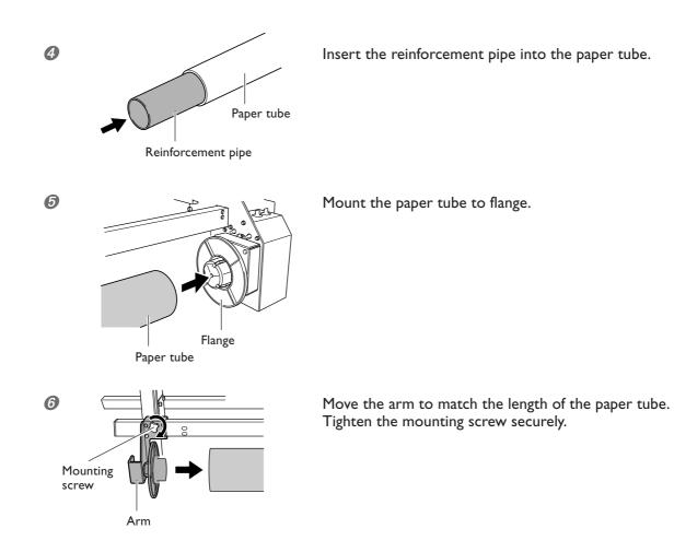
$I_{\bullet}$  Load the media onto the roll shaft.
