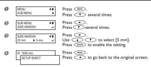
Choosing "5 mm" at this menu reduces the left and right margins, expanding the printing area. "20 mm" sets the margins for the printing area at 20 millimeters.
