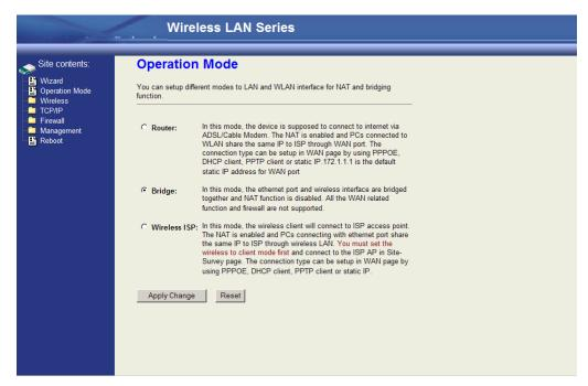
First under Operation Mode, make sure both units are in 'Bridge' mode.
