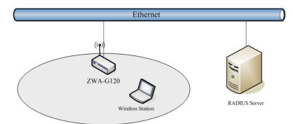
You should choose WEP 64 or 128 bit encryption based on your current network requirements. Then add user accounts and the target device to the RADIUS server. In the device, you need to specify the IP address, Password (Shared Secret) and Port number of the target RADIUS server.
