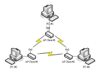
In client mode, the device can not support the Router mode functions including Firewall and WAN settings.
