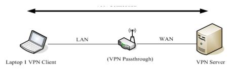
This functionality lets the device Pass-through the VPN packets including PPTP/ L2TP/IPsec VPN Connection.
