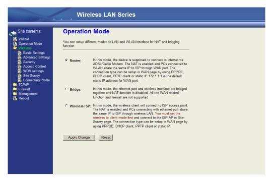
To enable the Access Point with routing, first change the Operation Mode to 'Router'.
