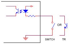
External inputs are interlocked with the touch keys.
