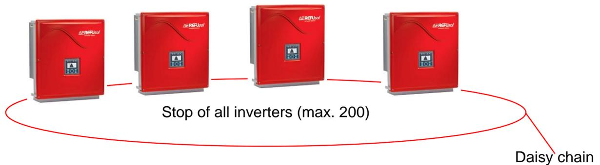
Figure No. 31 External shutdown signal within the "daisy chain"
