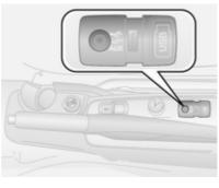
In the centre console there is an AUX socket for the connection of external audio sources.
