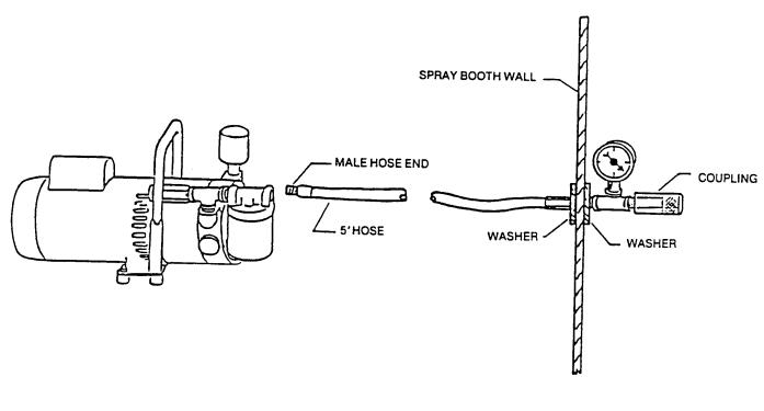
**CAUTION:** AIR SUPPLY PUMP MUST BE PLACED IN A "CLEAN-AIR" ENVIRONMENT WHERE BREATHABLE (GRADE D) AIR CAN BE ASSURED AT ALL TIMES.
