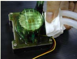
Joint between Water Block and water tubes
