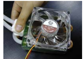
Joint between the radiator and water tubes
