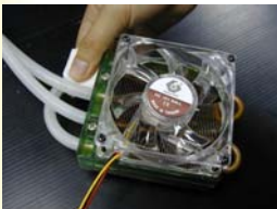
The U-shaped water tube outside the radiator
