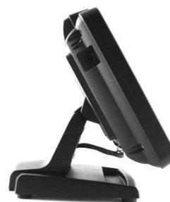
software resource conflict a simple push on the switch may fail to turn off the power. In this case, please utilize the **forced power off feature** by pressing the switch and holding for within 10 seconds.
