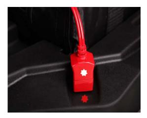
With the Star on the Battery lead aligning with the Star on the Battery tray, push down on the lead until the connection is fully made and the plug will not go down any further, as per the photos.
