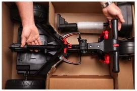
Place your hands on the buggy as per the photo and lift upwards to remove the buggy from the box.
