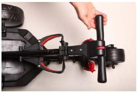
Lift the top section of the handle until the main handle assembly is full extended and laying down as per the photo below.
