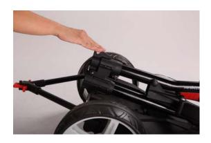
Lay the rear support section of the handle down and ensure that the folded handle is completely lowered down into the Battery Tray, as per the photo.
