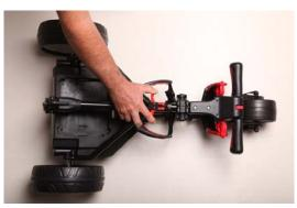
On the top of the buggy, you will see two Red Levers, which lock the frame into the folded position.
