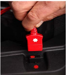
Connect the Battery Lead attached to the battery, onto the power connection of the buggy, as per the photos.
