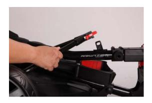
Lift and fold the rear support section of the frame which houses the two Red Levers, until it meets with the folded handle, as per the photo.
