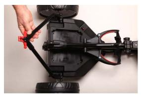
Press either one or both of these Red Levers to release the frame lock and lift the rear support section of the frame until it is laying down, as per the photo.
