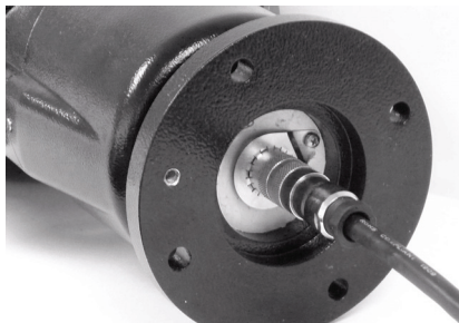
Figure 3.7 Composite cable connected to a MIC camera
