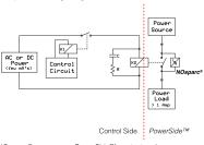
NOsparc® suppresses PowerSide™ contact arcing.
