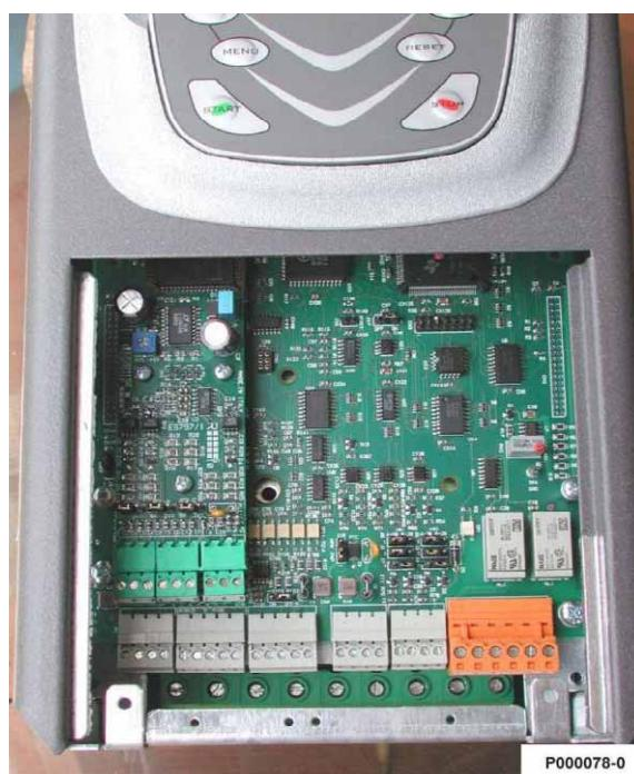
Figure 79: Encoder board fastened to its slot.
