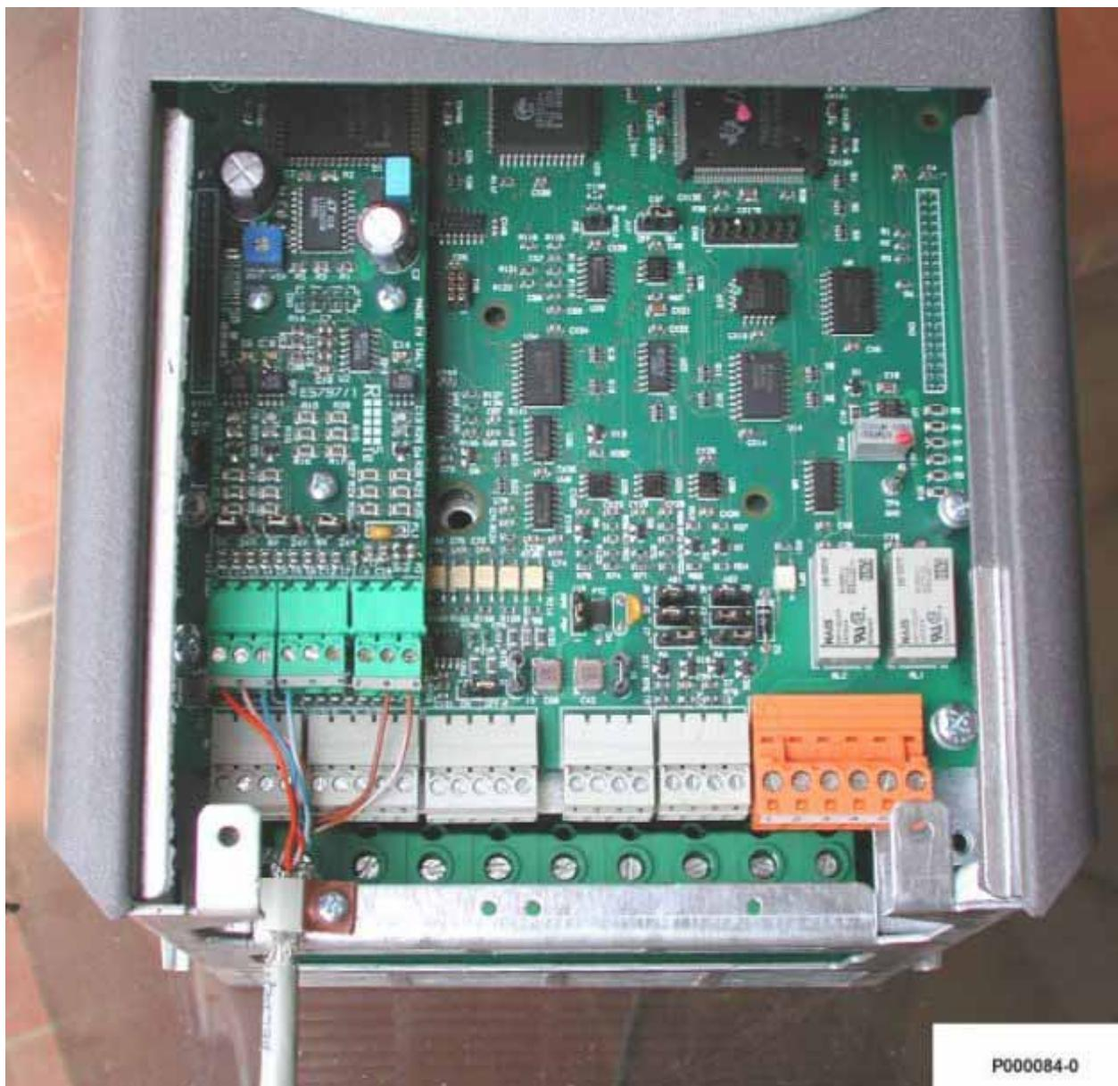
Figure 85: Wiring the encoder cable.
