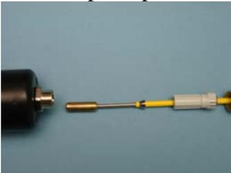
Screw on (finger tight) the new Staff while griping the metal rod
