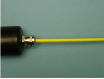
Unscrew the cord grip cap and slide out the plastic insert
