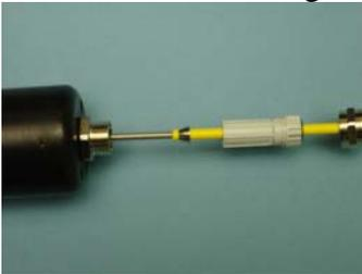
Unscrew the Staff while gripping the metal rod. Do not use any tools to clamp onto the yellow portion of the staff as this will damage the Teflon cover.
