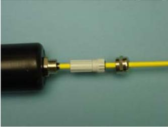
Slide the Teflon tubing back to access the metal rod
