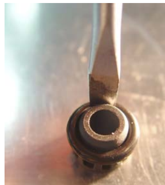
O-Ring in correct position
