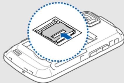
3. Lift the memory card cover and insert a memory card with the label side facing up.
