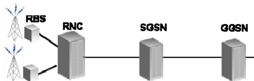
IP packets are sent in packet switch data channels over the radio network. To increase the success rate of fax calls it's important to have a connection with as little as possible latency and jitter since, despite T.38, Fax devices are sensitive to timing. WCDMA is a minimum requirement, but it's recommended to have a HSPA connection since this reduce the latency and jitter. Future radio network improvements, mainly regarding QoS, the fax transmission success rate will further improve.
