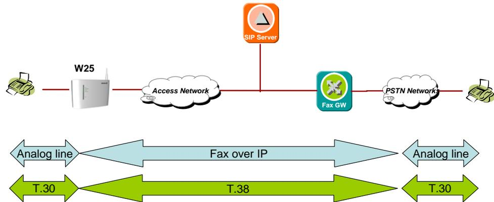
**Figure 1** - Typical network for VoIP running Fax (T.38)
