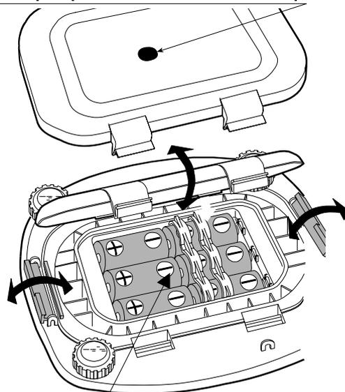
New six batteries. (R20P/ LR20/ D size)
