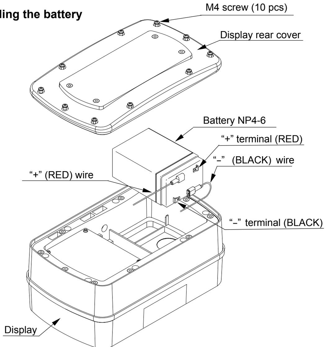
1. Disconnect the AC power cable from the electrical outlet.
