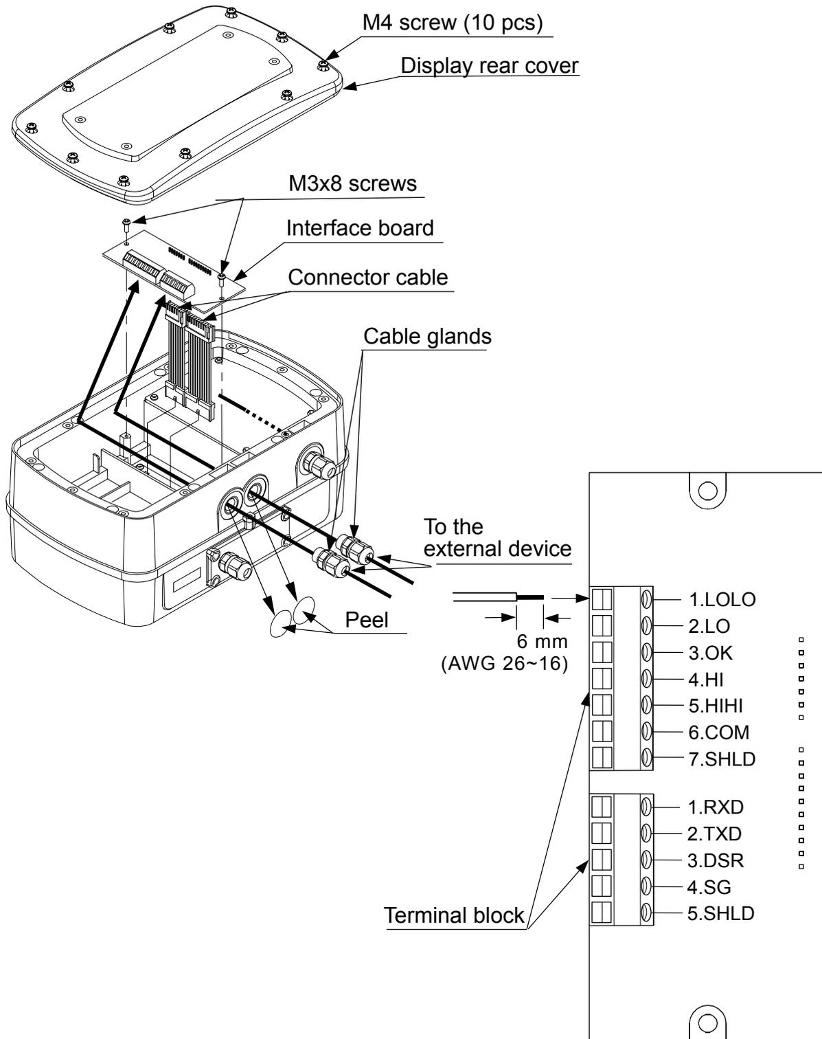
1. Disconnect the AC power cable from the electrical outlet. When the battery is installed, make sure that the scale is turned OFF.
