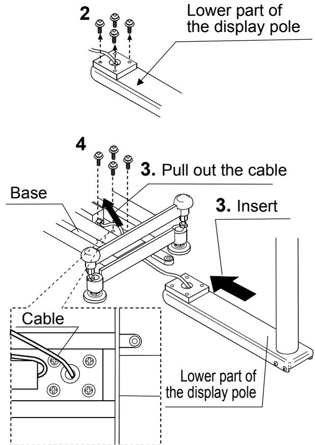
5. Lay the base on its side. Remove the 4 screws ("5" in the illustration) and remove the pole support foot.
