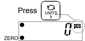
2. Press the **SAMPLE** switch to enter the sample unit weight storing mode. The numerical value on the left indicates the number of samples.
