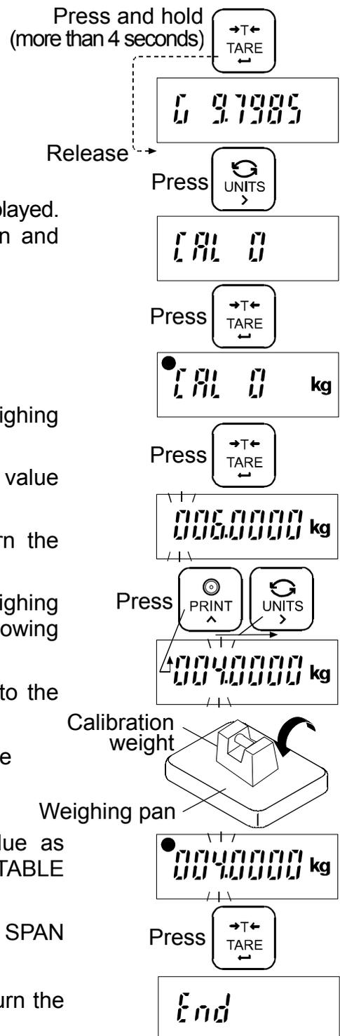
**Note:** If the scale will be moved to another location, set the gravity acceleration value for the new location and calibrate the scale according to the procedure above. Refer to the previous section to set the gravity acceleration value.
