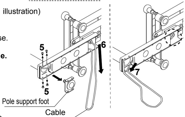
8. Put the bundle of cable back into the display pole. (See "8" in the illustration.)
