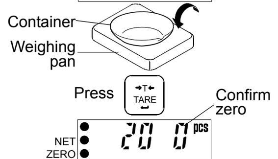
5. Place the correct number of samples on the weighing pan or in the container.
