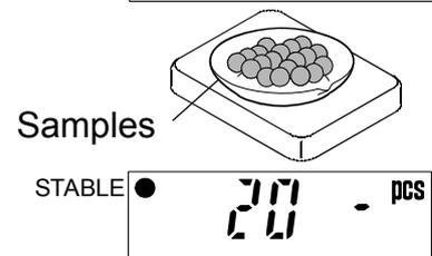
□ The total weight of samples should be more than shown below, regardless of the number of samples.
