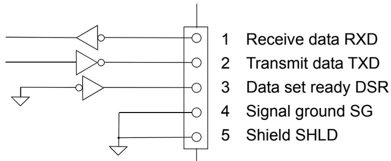
❑ SW is designed as DCE (Data Communication Equipment).
