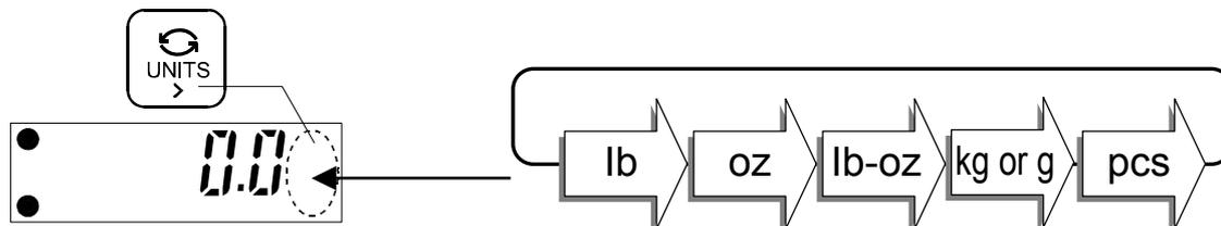
Using the function setting “ $U_t - G$ ”, “kg” and “g” can be switched.
