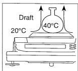
Operate your balance gently. Shorten the operation time as much as possible (Opening and closing door, placing and removing material). Use a pair of tweezers (pincette) to avoid temperature changes due to heat from inserting your hand into the weighing chamber.
