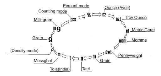
If a mode (or unit) of weight has been turned off, the sequence will be missing that mode or unit. There are also the various Tael that can be included if necessary. (Tael is selected as a unit from four units installed at the factory)
