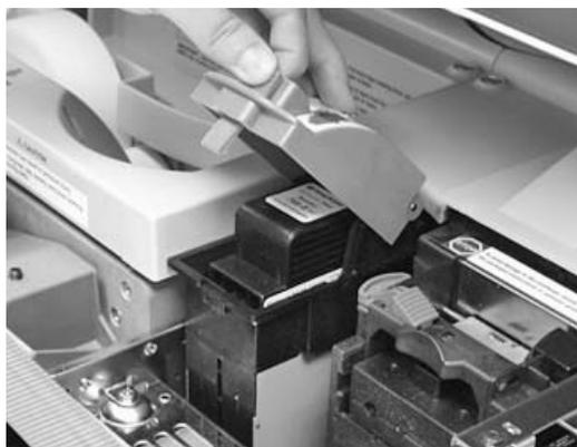
3. Remove the old ink cartridge by lifting it straight up.
