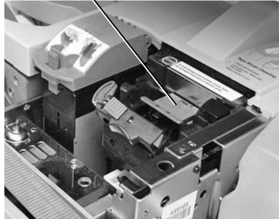
6. Grasp the printhead cover and pull as shown here.
