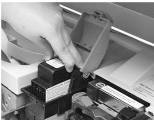
4. Insert the new cartridge with the grooved side facing you.
