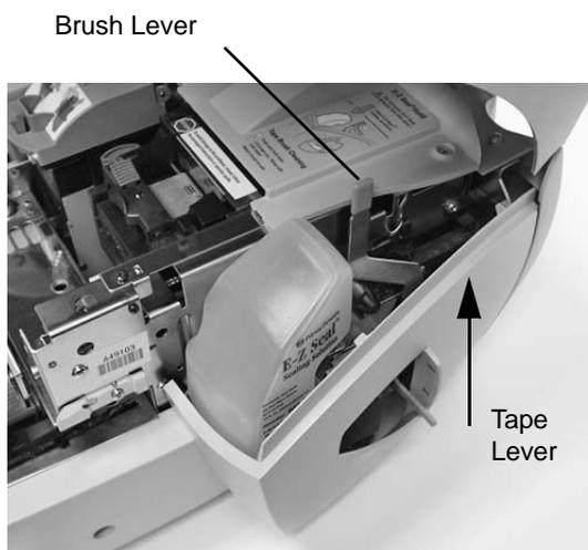
5. Place the brush in the case, two or three teeth away from the bottom. The shorter bristles should be against the solid side of the holder.
