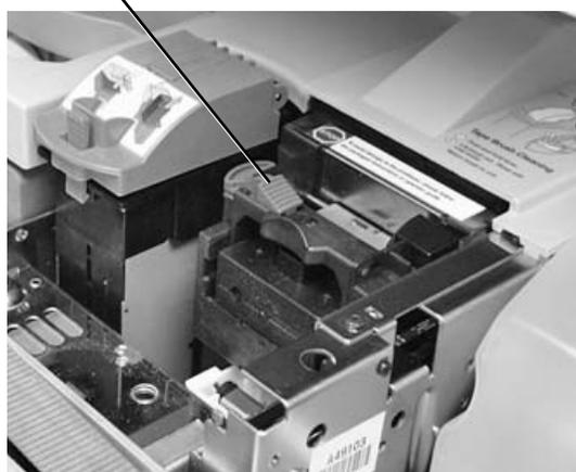
5. Push the printhead tab to the left. While continuing to press the printhead tab to the left, pull the assembly forward as shown here.
