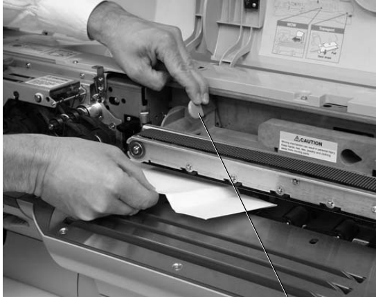
WOW® transport jam release lever
