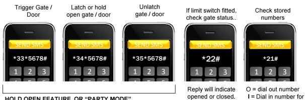
HOLD OPEN FEATURE, OR "PARTY MODE" Some gate systems allow hold open control, depending on manufacturer. Send the following SMS commands to control the gates..
