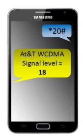
Note: Reception levels below 14 can give problems with the relay operation, and poor or no audio coming from the microphone on the intercom (the person on the phone cannot hear anything)
