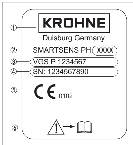
Figure 2-3: Example for a nameplate on the sensor body
