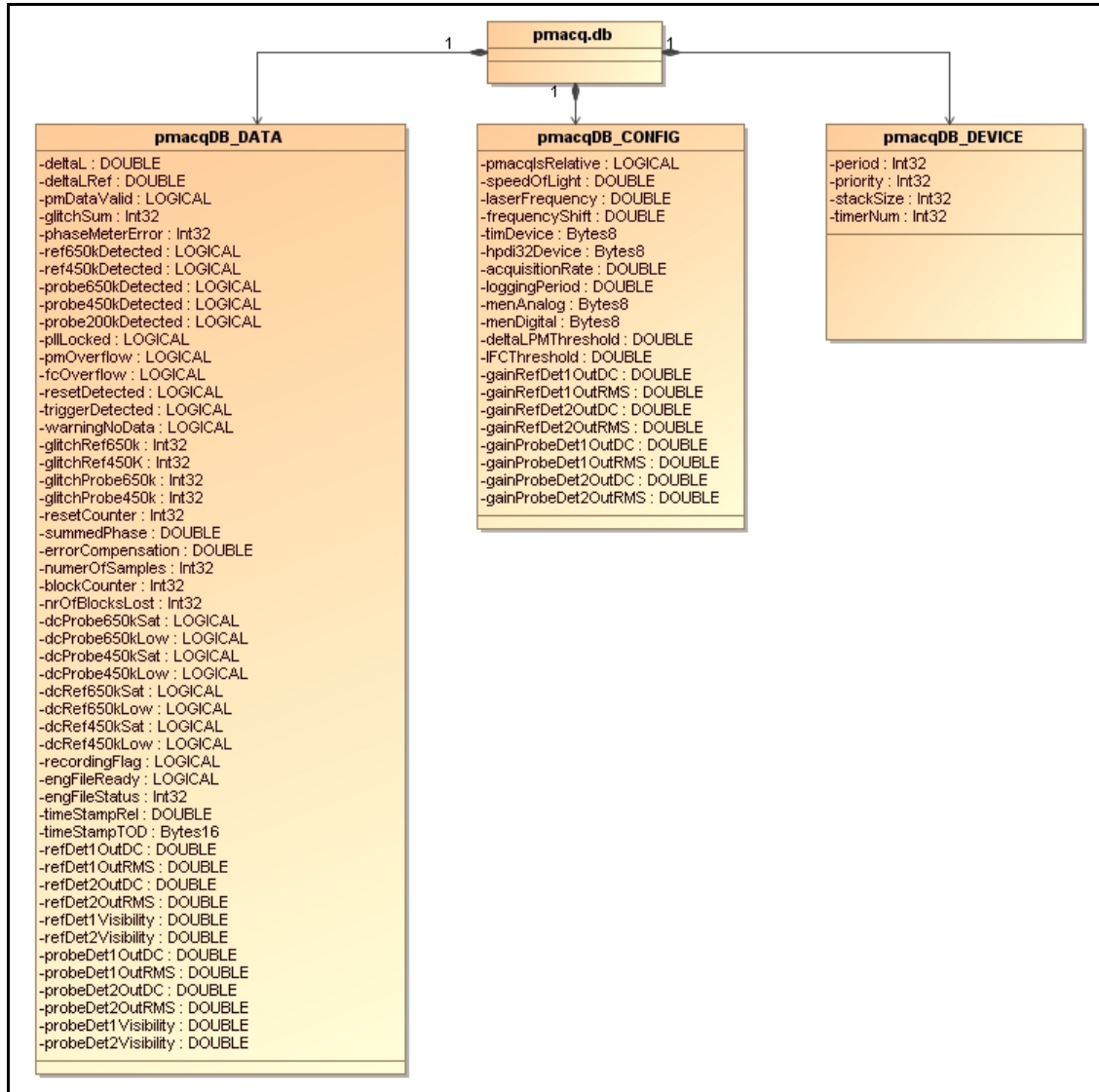
Figure 15: PMACQ OLDB Structure
