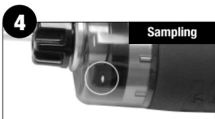
**Draw the sample gas.** Take a sample for the specified time at the desired sampling point as shown in the tube instructions. The sample is complete when the flow finish indicator appears.
