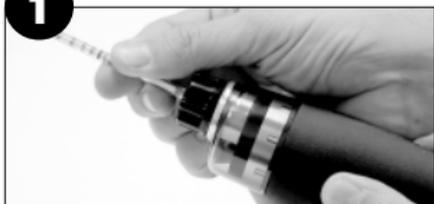
Insert a **sealed, unbroken detector tube** into the rubber tube connector. Align the red lines on the pump and shaft handle, and pull the handle to full stroke locked position.
