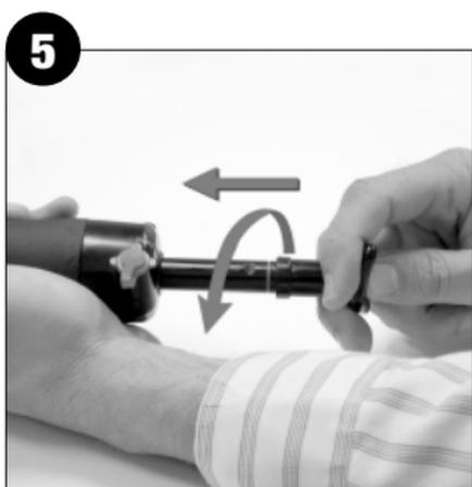
**Return the handle.** When the sample is complete, turn the handle 1/4 turn (90°) to unlock the handle. Confirm that the handle remains extended. (If the handle returns part way, the sample is incomplete, causing a low reading). If the detector tube requires more than one stroke, push back the handle and repeat the operation, as many times as required.
