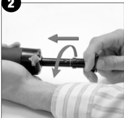
Wait one minute. Unlock the handle by turning it 1/4 turn (90°). Hold the cylinder and handle **securely** while allowing the handle to **slowly** return to its initial position. The pump passes the leak test if the handle returns completely to its original position. If the red line on the pump shaft is visible, the pump has failed.
