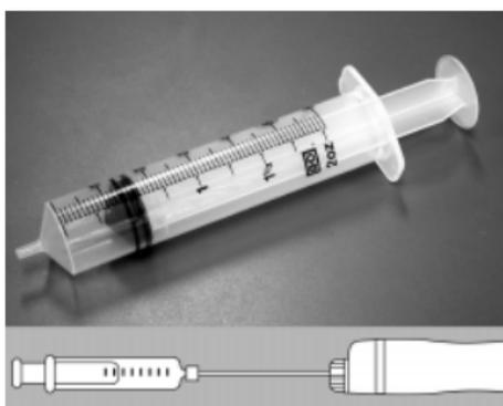
50cc of sample gas into a 100cc syringe. Complete the syringe draw with fresh air. Take a reading and multiply by 2.
