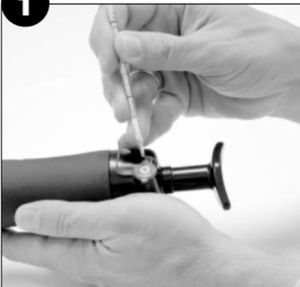
**Cut both ends of the detector tube.** Insert the tip of a fresh gas detector tube into the tip cutter. Score the tip by rotating the tube one revolution. Pull the tube toward you at an angle to break the tip.
