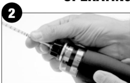
**Insert detector tube.** Insert the gas detector tube into the rubber tube connector in the pump. Make sure the tube's arrow is pointing toward the pump.
