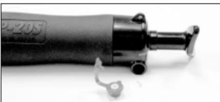
(The glass tip can be disposed by removing the tip cutter cap.)
