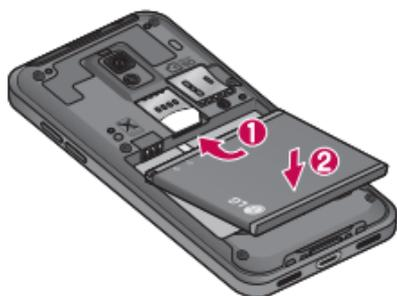
4. Align the back cover over the battery compartment (1) and press it down until it clicks into place (2).
