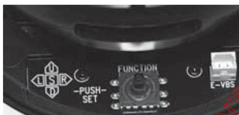
In order to enter the menu press the joystick, which results in executing **SET** command. For choosing the submenus please move the joystick into **UP**, **DOWN** positions. If a **↵** symbol is present, enter particular sub-menu by pressing the **SET** button. To change the parameters use the **LEFT** and **RIGHT** joystick positions.
