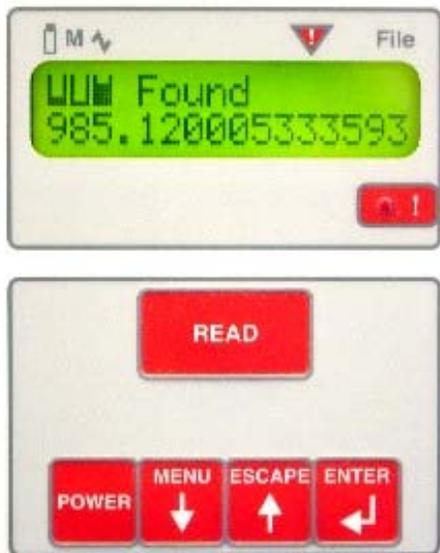
**STEP 9:** The Red LED will blink and the Pit Tag Code will be displayed. The detection system is now "tuned" and ready to configure\* for use.
