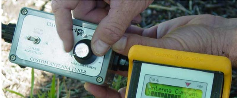
**STEP 4:** Adjust the fine and/or coarse adjustments on the antenna tuner until maximum current is displayed on the FS2001 reader. (Coarse adjustment is generally not required.)
