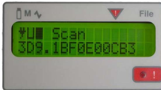
**Figure 3 Tag Code in Reader Display**
