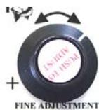
**Slowly** adjust the "Fine Tuning Adjustment" not more than 1/16th of a turn in either direction. Then wait 3 to 5 seconds to allow the reader display to catch up with the tuning adjustment. When current reaches maximum, further adjustment in the same direction will cause current to decrease. Simply tune back to the maximum current setting.
