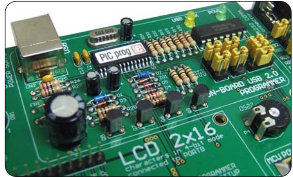
Figure 10. USB programming connector
