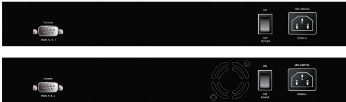
Figure 4: GE-DS-82 and GE-DS-82-PoE Rear panels
