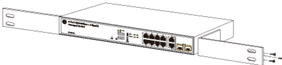
Figure 6: Attaching rack-mount brackets to the GE-DS-82
