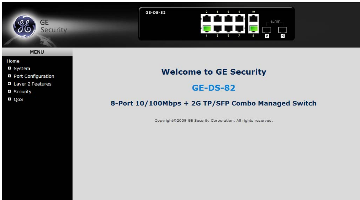
Figure 12: Web main screen of Managed Switch
