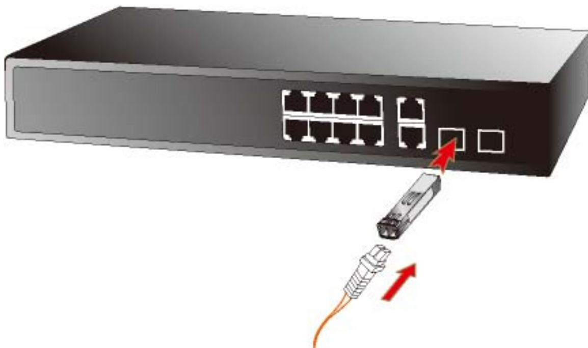
Figure 8: Plugging-in the SFP transceiver
