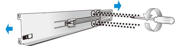
**2-3. Attaching the rails to the rack posts**
