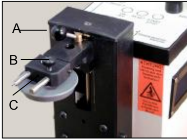
Fig.3 Adjustment of the upper tank holder
