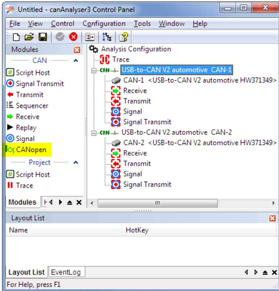
Figure 2.1: Control Panel with CANopen-Module
