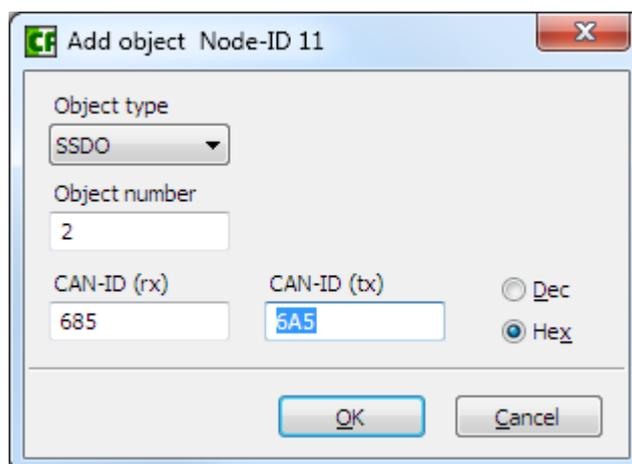
Figure 3.8: Add CANopen communication object (e.g. SDO)
