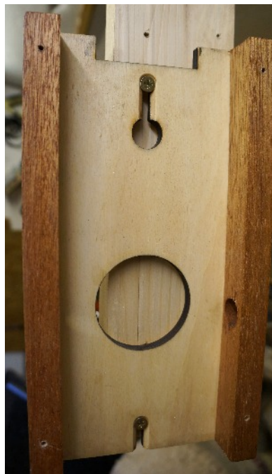
Wall plate removed from clock to show wall mounting screws just below the surface.
