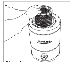
Step 4 First remove HEPA filter by placing your hand on the inner side of the filter. Then pull up gently until totally out.
